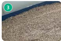
③ Recycling of metal scraps generated during the cutting of wheels and the production of molds, jigs, tools and the like
