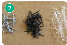
② Reuse of runners discharged during plastic molding
